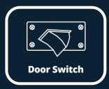
Our A-Fit cabinet combines functionality and outstanding energy performance to meet Japanese quality standards, with precise temperature control to ensure food-ingredient freshness at all times. With the R290 natural refrigerant and a door switch preventing the evaporator fan from running while the refrigerator is open, they not only perform efficiently but also support a greener tomorrow.
